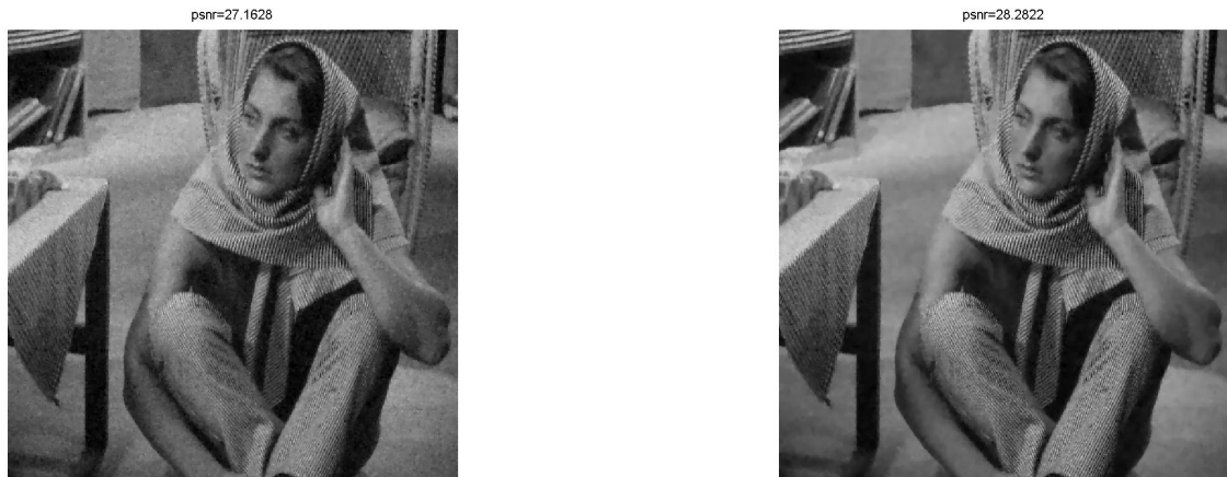
FIG. 5.2. The denoised images by the PM method and the denoised image (right) by our finite difference scheme
