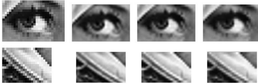
**Figure 5.** Two images are scaled by a factor of 10 using the MSA spline method with  $d=7$  and  $r=1$ . The results are compared to the bicubic and bilinear interpolation methods implemented in the MATLAB®'s function `imresize`.<sup>53</sup>
